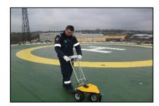
Findlay Irvine are world leading experts in measuring skid resistance for airports having been manufacturing Continuous Friction Measuring Equipment (CFME) for over 20 years. Currently in use in over 550 airports worldwide, GripTester MK2 is the world's most versatile, robust and deployable continuous friction measuring device. Also now available is the micro GripTester for Holidacks
