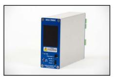
The **Findlay Irvine** Data Collection Unit DCU390-C is a data logger for use in Remote Condition Monitoring applications for track assets. The DCU390-C has been designed to meet and exceed Network Rail's current data logger standard The (NR/L2/SIF/30036). unit is fully compatible with Network Rail's data logger standard (NR/L2/SIG/30036) and Intelligent
